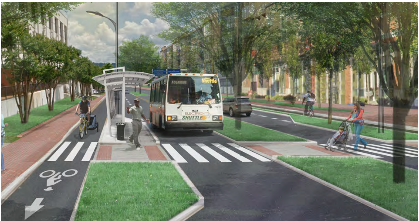
Example of a Complete Street design that accommodates many uses such as walking, biking, driving, and transit.
