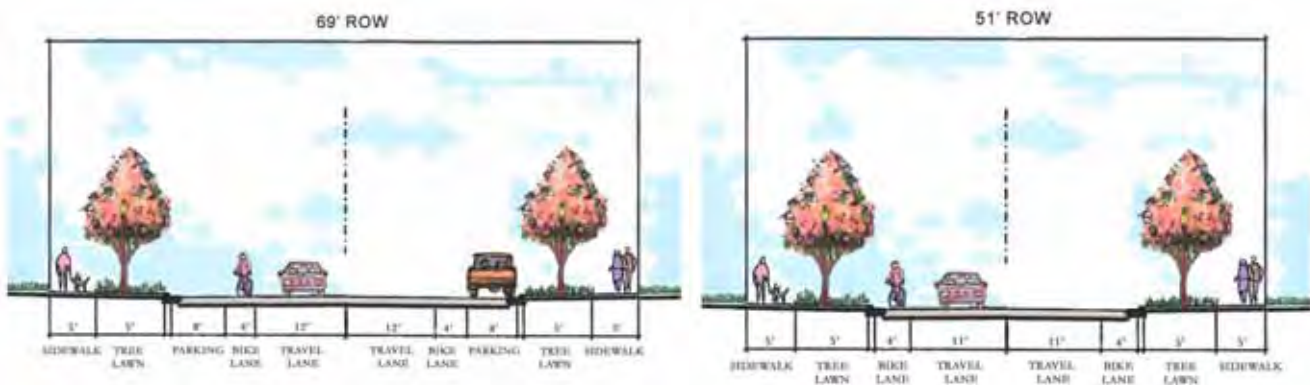
Typical collector street cross sections (with and without parking) (not to scale)
